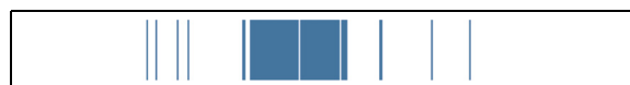
Fig. 7. Position of similarity between PCAP-file and installer file in reference set indicating that the file was transferred in the middle of the traffic recording session.
