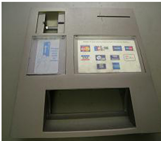
Fig. 3 – Imitation ATM fascia – front and rear view.
