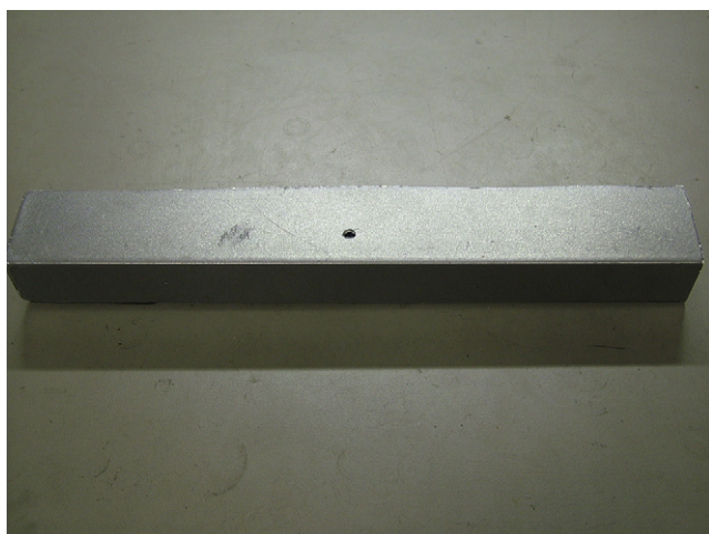
Fig. 6 – Front face of plastic strip containing a small pinhole for the camera lens.
